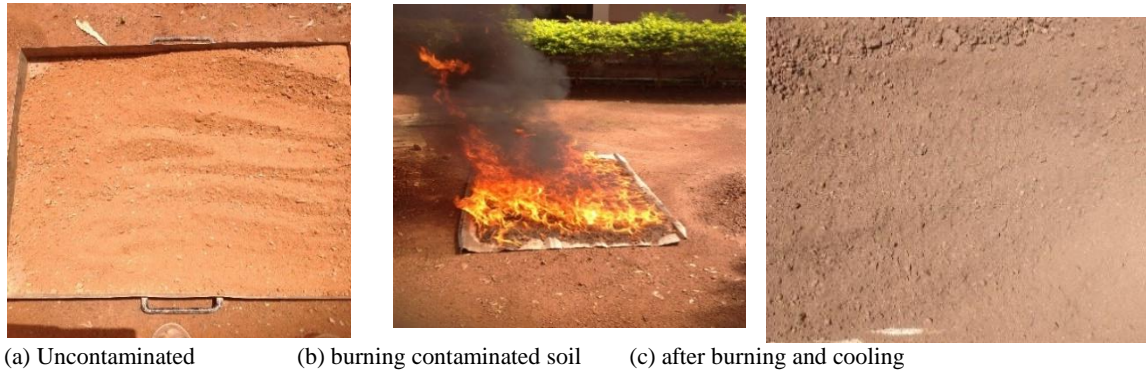
Fig. 2: Crude oil contamination and burning process
